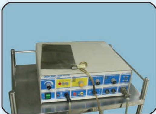
Photo-18. Cautery: The patient plate should be in contact with maximum surface area on the patient. Do not use wet cloth, jelly etc for this.
