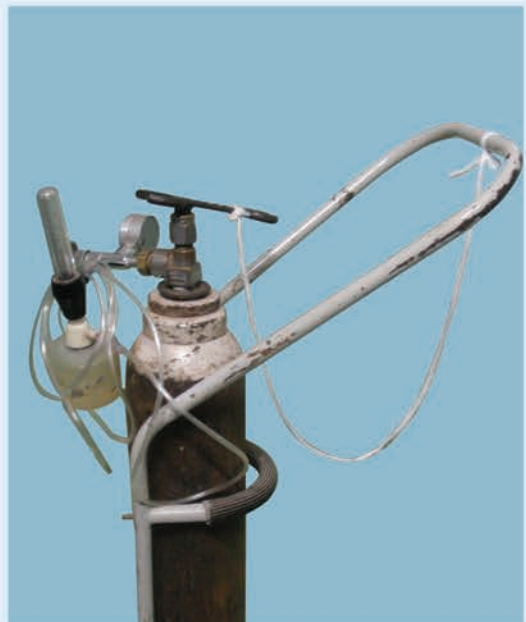
Photo-14. The spanner should be tied to the oxygen cylinder. The water in the humidifier should be changed daily and the date should be marked on it.
